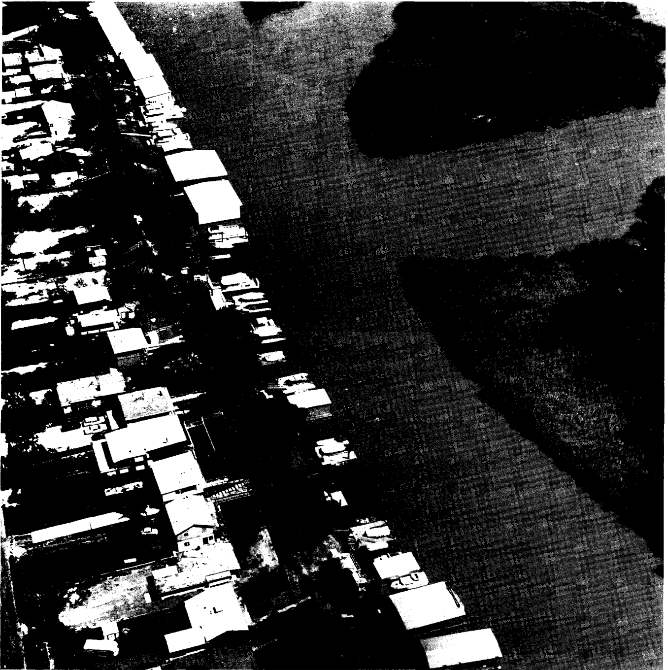
Urban development is increasing as the desire to live near water draws people to the Delta. Houses, docks, and other structures obstruct inspections and maintenance of levees. Many Delta levees do not meet minimum criteria for protecting urban development.
